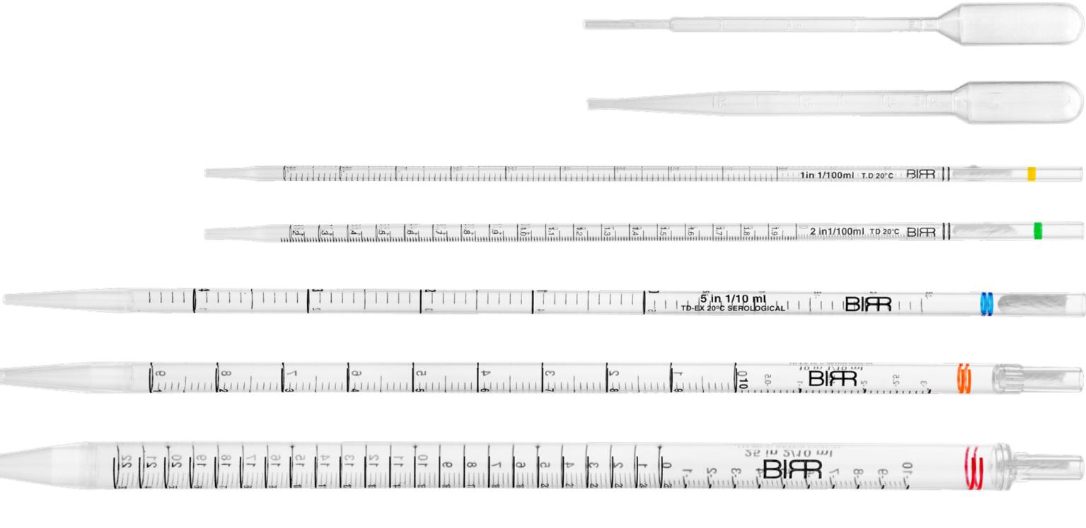
• Dropping pipettes are made of medical-grade Polyethylene (PE) • Serological pipettes are made of medical-grade Polystyrene (PS)
